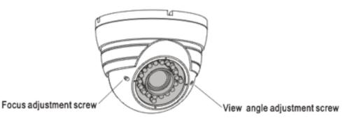
Make sure the ring is firmly tightened before and after adjusting the lens.
