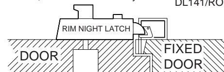
Fitting arrangement for rim night latch & rim electric release to a double outward opening fully rebated door.
