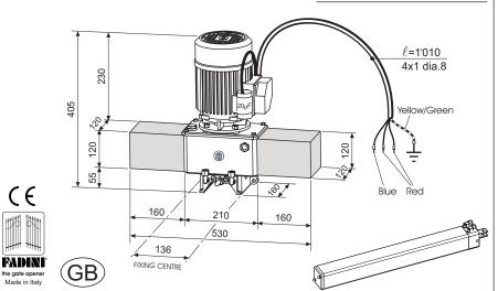
"MEC 800" **400 mm stroke** is an electro-hydraulic operator designed to open/close solid panel doors of 3m up to 5 m width and trap doors of large dimensions.
