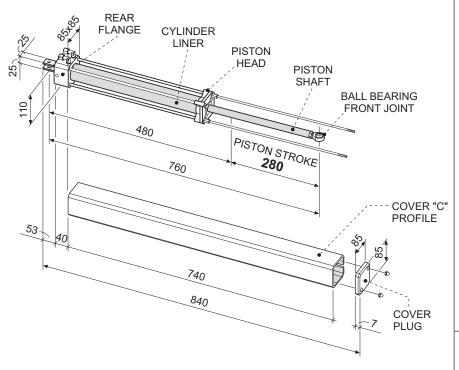
"MEC 800" is an electro-hydraulic operator designed to open/close solid panel doors and trap doors of large dimensions. By means of its dual structure, ie. motor pump assembly and ram operator, it can electrically operate gate weights from 450 Kg up to 600 Kg. Where heavier rating is required, it is possible to install two rams with one double-tank motor pump on each gate leaf, to operate gate weights of 500 Kg up to 700 Kg.
