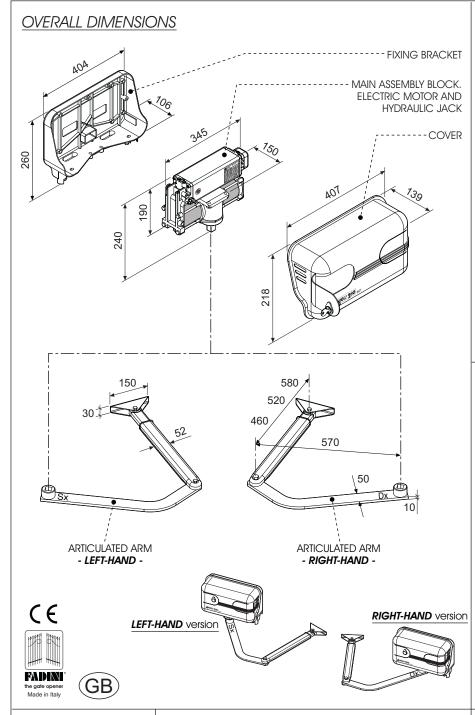
"APROLI 280/700 STRONG" is an oil-hydraulic gate operator designed for swinging gates hinged to large pillars.
