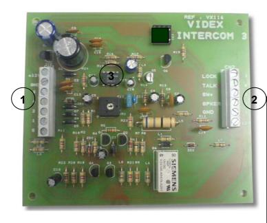
The intercom 3 apartment station interface PCB is required whenever the 500, 500M or 500ST apartment station are used. This PCB converts the duplex speech into simplex speech and controls the switching of the apartment station
