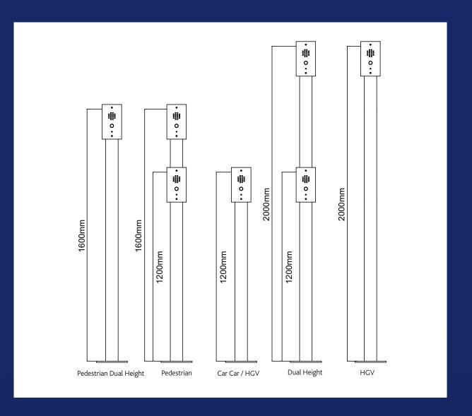
All Post are manufactured from 80mm  $\times$  80mm brushed Stainless steel and incorporate a substantial 200mm  $\times$  200mm  $\times$  8mm base plate with 4  $\times$  14mm diameter fixing holes to secure the unit.
