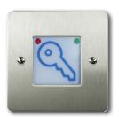
The PN4RF reader fits into a standard single gang flush box. Available in brushed or mirror polished stainless steel Dimensions H 85 W 85 D 30
