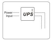
The electromagnetic lock is failsafe and will require a power supply unit equipped with battery back up for fear that power failure may increase security risks.
