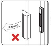
Installing the maglock on outswing doors/frames will pose security problems.
