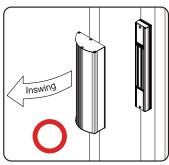
Notice that PH-450/PH-900 series of maglocks should be installed on "inswing" doors and frames for the sake of security.
