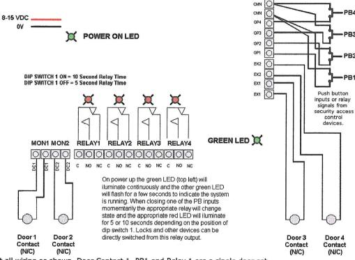
Connect all wiring as shown. Door Contact 1, PB1 and Relay 1 are a single door set.
