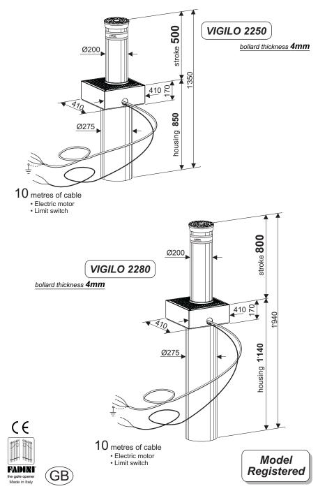
**VIGILO** is an electro-hydraulic post for traffic control. The motor pomp is incorporated and pre-connected. This makes the unit easier to install. The cylindrical post is made of steel, has a diametre of 200 mm and can be commanded to rise from the ground level or lower by remote control.
