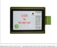
Interface that enables local connection between the PC (USB port) and the installation, to configure, control and manage the facilities. Used for maintenance of facilities that do not have the PC permanently connected, as an installer tool.
