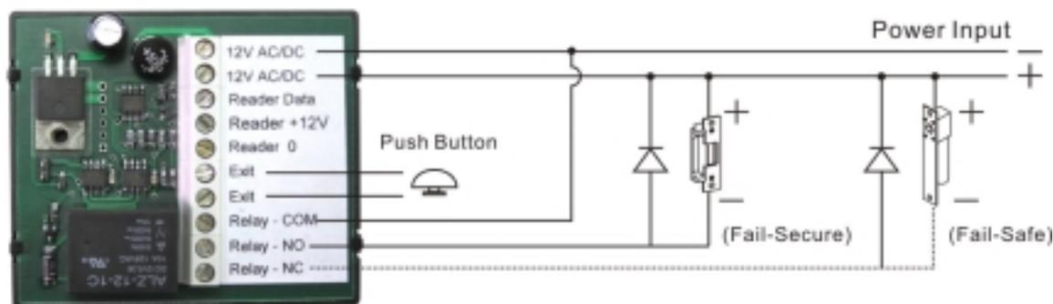
Note: When using a strike with DC, the relay contacts will be damaged by arcing due to back EMF when the contact opens. Use a IN4001 diode as shown on the drawing to prevent this damage.
