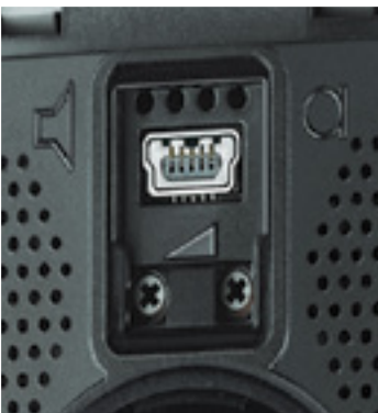
Mini-USB connection and loudspeaker/microphone volume adjustment
