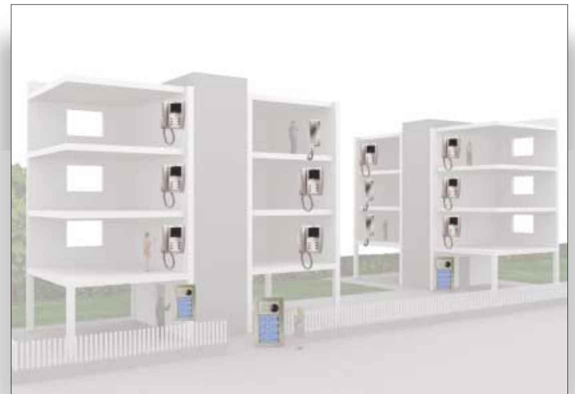
Several communications from main and secondary entrances are possible at the same time.
