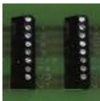
Simplewire connection board for connections including speech, lock release, ground, video power and the call line
