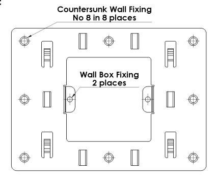
**Warning.** The heads of the countersunk screws must protrude less than 1mm or there will be difficulty attaching the apartment station to the plate.
