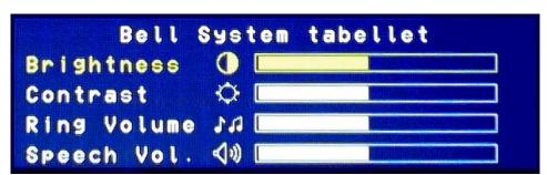
When adjusting the ring volume a short ring is given each time it is increased or decreased to give an audible indication of the volume.
