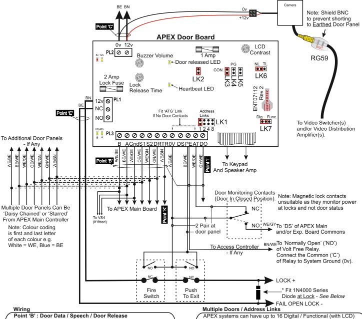
6 Pair CW1308 - Any unused cores to be tied to system ground
