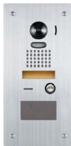
JK-DVF-HID* PTZ video door station, stainless steel, flush mount with HID® ProxPoint® Plus embedded card reader W: 5-3/4" H: 11-5/8" D: 1-3/4"
