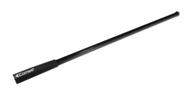
Wireless active infrared barrier with a range of 5 m guaranteeing the utmost active efficacy in detecting the crossing of an access point or perimeter, thanks to the use of constantly monitored pulsed beams. Protected beam height: 2 m. Batteries inside the trim to enhance the compact dimensions. Dimensions:  $40 \times 2220 \times 40$  mm.
