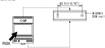
Mount DIN rail to wall board inside an electrical enclosure. Attach PS-2410DM to DIN rail aligning at the hook and pushing bottom until it clicks to lock.
