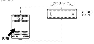
Mount DIN rail to wall board inside an electrical enclosure. Attach PS-1820DM to DIN rail aligning at the hook and pushing bottom until it clicks to lock.
