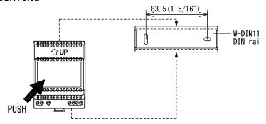
Mount DIN rail to wall board inside an electrical enclosure. Attach PS-1225DM to DIN rail aligning at the hook and pushing bottom until it clicks to lock.
