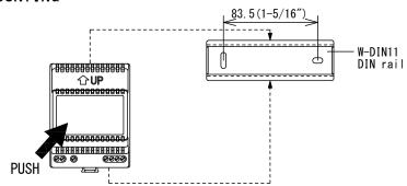
Mount DIN rail to wall board inside an electrical enclosure. Attach PS-0602DM to DIN rail aligning at the hook and pushing bottom until it clicks to lock.
