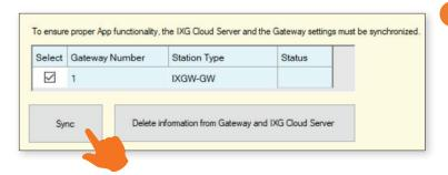
If the sync fails, or the status LED never turns green, confirm both the programming PC and the Gateway have an internet connection. Also, confirm the Default Gateway and DNS settings configured under **Network Settings** are set correctly.
