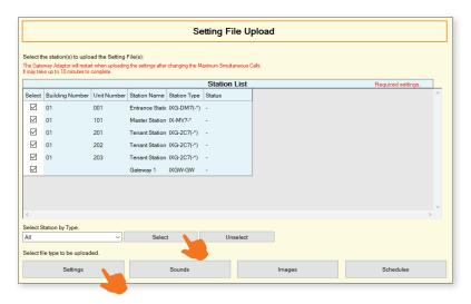
If any stations fail, they may still be booting up from the Association Settings step. It is also important to ensure that the programming PC is in the same subnet range as the stations. For example, if the stations are set to 192.168.1.xx, the PC should also be set to this.
