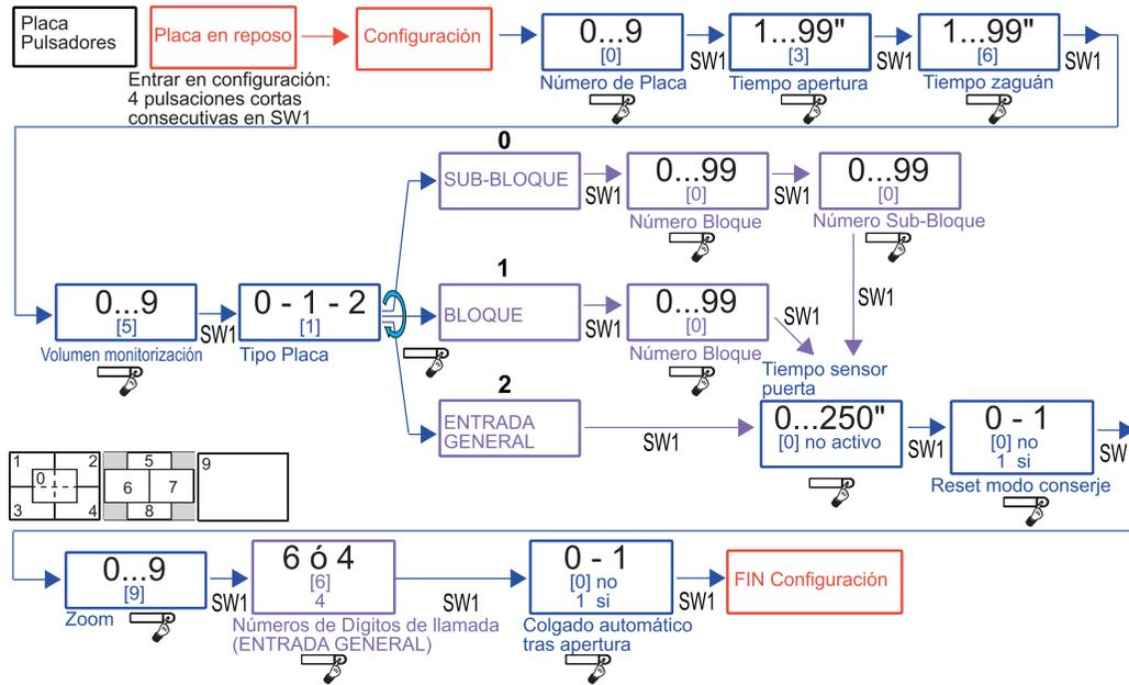
ANNEX: ASSISTED CONFIGURATION BY VOICE IN PUSHBUTTONS PANELS
