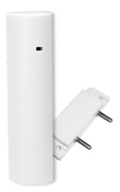
RFH2O is a wireless flooding sensor that detects the presence of water at ground level. It comes with an adjustable sensor that connects to the transmitter via a cable that is 2 m in length.
