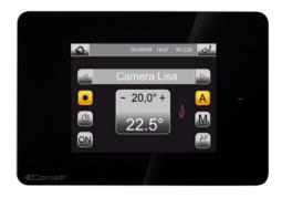
3.5&rdquo, Mini Touch with programmable thermostat function. For connection to the SimpleHome bus. Integrated temperature sensor, 1 switching relay output, 3 transistor outputs to control a 3-speed fan-coil. Yellow backlighting in accordance with thermostat status or with adjustable colour steplights function. Can be fitted in a 3-module wall box for civil series.
