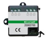
SimpleHome BUS separator/regenerator module. Enables you to isolate and regenerate the bus in systems with more than 40 modules. For direct connection to the SimpleHome BUS, creating islands with max. 40 modules. Possibility to separate only the BUS or also the power supply.
