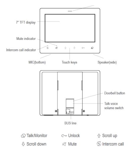
Talk voice volume switch: the volume of the speaker voice when talk with door station, up means high, down means low.
