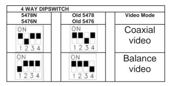
Connections, 8 way dip-switch bank, programming, and functions are the same as the 5478/5476 with the exception of the "??" button which is non-latching on the 5478N/5476N. The "Def" button is also used instead of the "??" button when programming the call tone melody.
