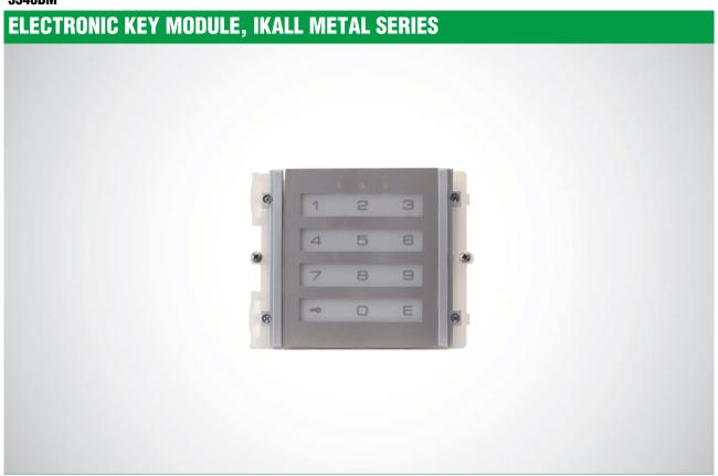
Digital electronic key module with LED keypad backlighting. Blue, white and off lighting options; stainless steel finish. When a number with between 1 and 8 digits is entered on the keypad, two relays (10A) are activated, allowing the operation of electric door locks or other devices. Dimensions 112x89.5x40 mm.
