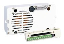
Speaker unit for 2-wire systems complete with terminal block and audio control with echocancelling, sealed-unit loudspeaker, electret microphone and front-mounted loudspeaker volume control. Complete with microprocessor and 8-position dip switch for programming calls to users. On-board electronic lock-release function (3A) plus C, NC, NO contacts for 10A relay. Timed lock-release input and door open indication. Compatible with power supply unit art. 1210. Dimensions: 102x55x38 mm.
