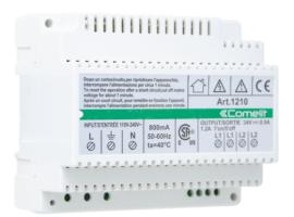
2-wire power supply unit required to power the external unit (terminals L1 - L1) and the support column (terminals L2 - L2). Equipped with 1 terminal for line termination art 1216. Input voltage 110-240Vac. Compatible with audio/video unit art. 4681 and 1621VC and audio unit art. 1621. Dimensions: 106x89x62mm (6 DIN modules).
