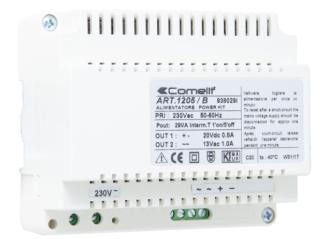
The transformer has 2 outputs: one to supply the external unit and the electric lock, and one to supply the monitor. 500mA delayed protection fuse.Terminal board:AC230V input mains voltage  $\sim \sim$  AC output for external unit and electric lock+ - 20V DC output for the monitor power supply. Dimensions: 105x85x85mm
