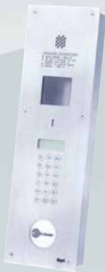
VRVD/200IMP 12swg stainless steel vandal resistant video panel with prox cut-out, 550hx165w front plate dimensions
